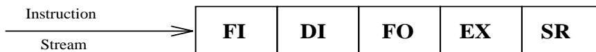
Figure 3: Pipelined execution of instructions. The steps are: FI, fetch instruction; DI, decode instruction; FO, fetch operand; EX execute instruction; SR store result. Since this pipeline has five segments, it can be operating on five instructions simultaneously. While the FI segment is fetching an instruction, the DI segment is decoding the previous instruction, and so on down the pipe.
