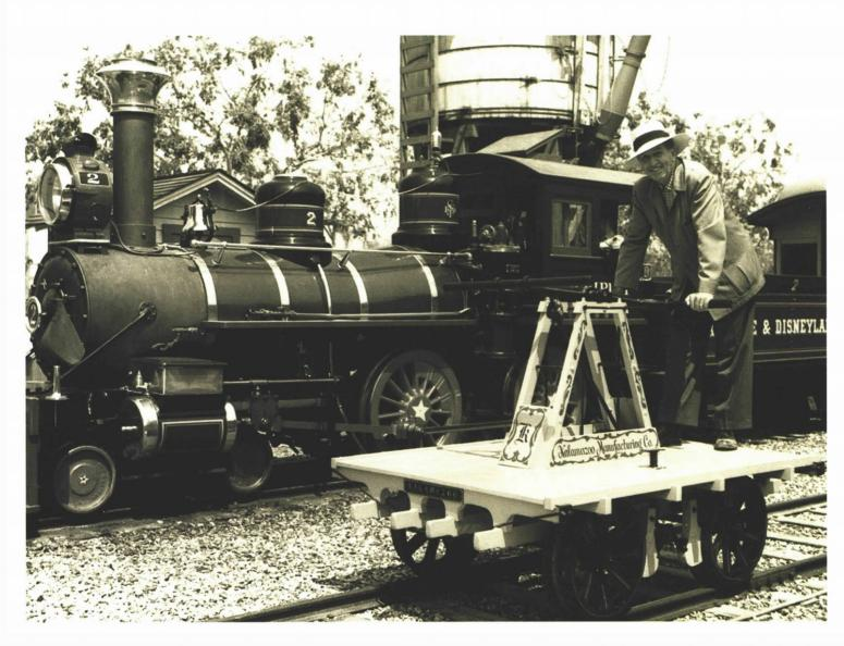
Walt tries out a Kalamazoo Manufacturing Company handcar on the Santa Fe and Disneyland Railroad. These "pump"-style, human-powered handcars, which translate the up-and-down motion of the pump into forward (or reverse) motion through gears, were once used by roving track inspectors and track laborers "commuting" to their work sites. © Disney Enterprises, Inc.
