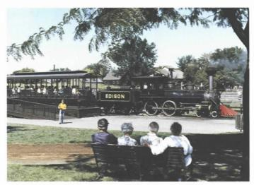
Above: Locomotive No. 1 "Edison" is rotated, by hand, on Greenfield Village's small turn-of-the-century turntable. Larger railroad turntables generally were rotated using compressed air or electric motors. © Henry Ford Museum & Greenfield Village.
