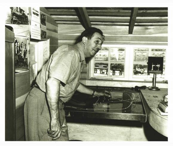
Walt "demonstrates" his Carolwood Pacific CTC dispatching board. Any of the railroad's 11 switches could be thrown electrically from the board, located inside the red barn, sending a train over a number of different routes. Progress of trains was monitored by tiny lights that would flick on, then off, as a train was "sensed" by track circuits along the route. Mrs. Walt Disney collection, © Disney Enterprises, Inc.
