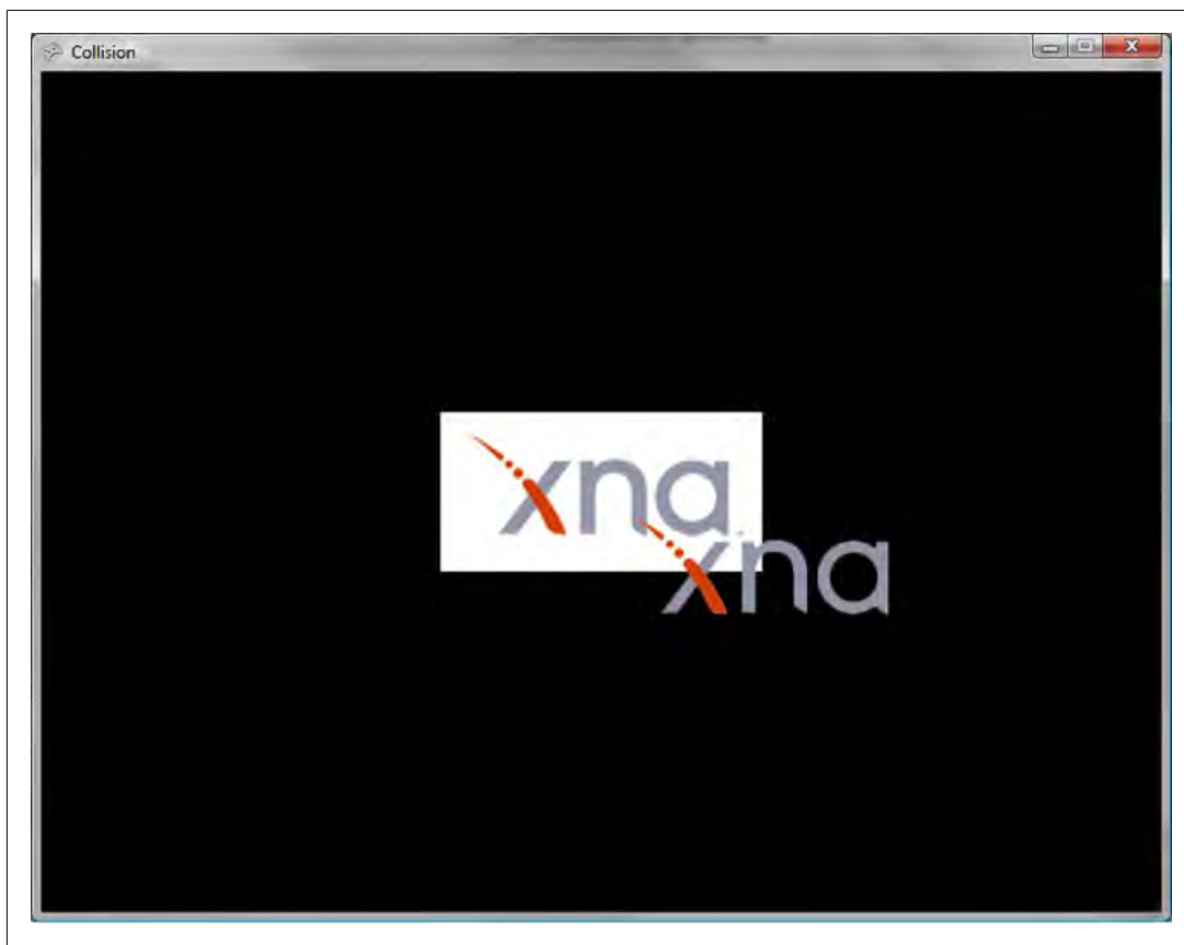
Figure 3-5. Two sprites, one with a transparent background and one without
